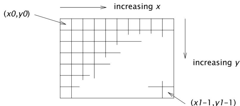
The picture file format described in *picfile*(9.6) is fairly simple. Such a *picfile* encodes a rectangular array of  $n$ -channel pixel records, each channel being a single byte. The file contains a textual header that describes the dimensions and encoding of
