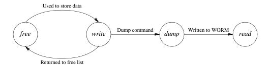
**Figure 1.** The state transition diagram for a block.
