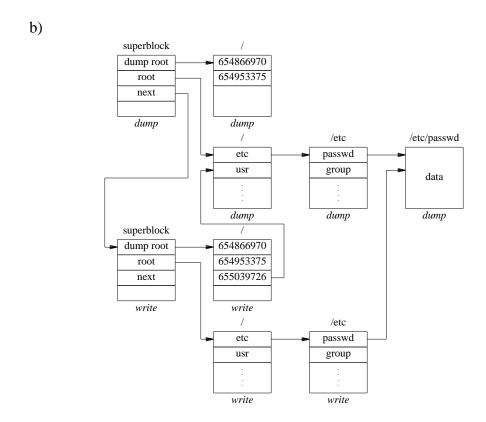
**Figure 3.** Before and after the dump command, assuming /etc/passwd is open.
