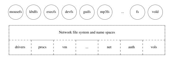
Figure 1: Architecture of the system software at a Plan B machine.
