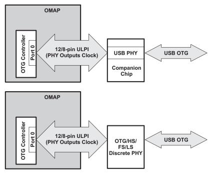
Figure 8. Typical Uses for USB Port 0
