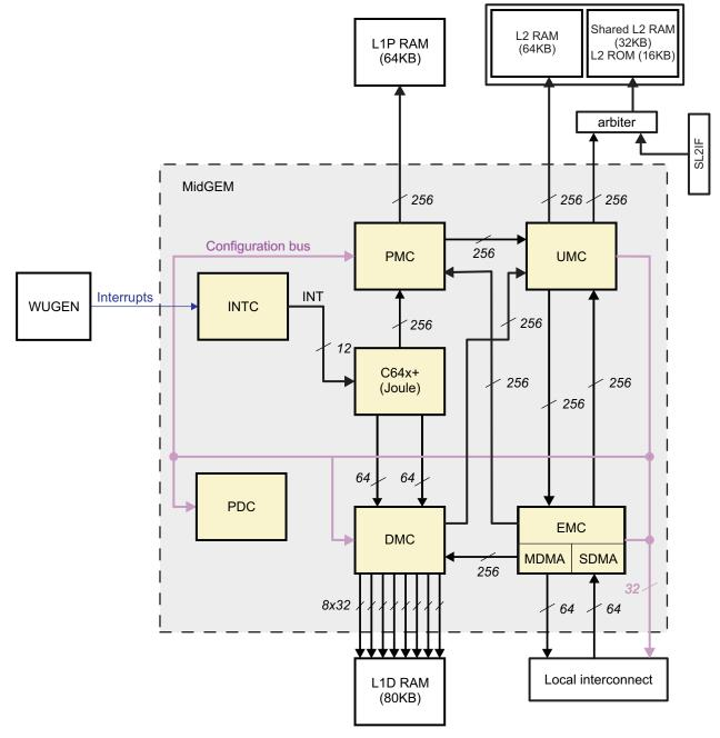
Figure 4. C64x+ Megamodule Block Diagram
