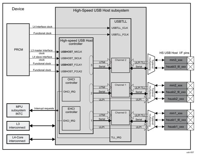
Figure 9. High-Speed USB Host Subsystem Highlight
